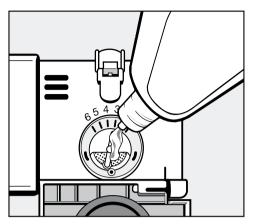
■ Pour liquid rinse aid into the reservoir until it is visible on the surface of the screen. Do not refill until the "Rinse Aid" indicator lights.
